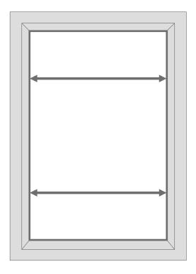
Take two measurements of the width, at the top and the bottom of the window.
